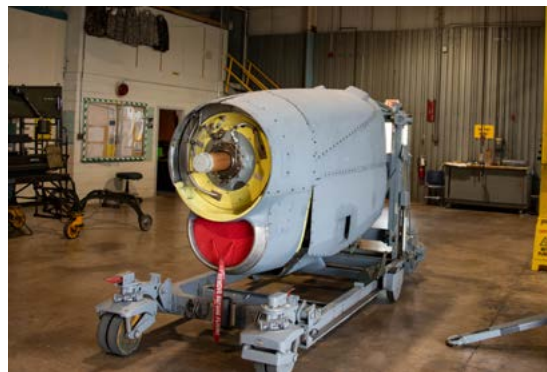
A T-56 Turbine engine waits to be married to a propeller and installed on a Delaware National Guard C-130H2.5 Hercules, 8-May-2022. A routine home station inspection revealed slight corrosion which made its replacement necessary. (U.S. Air National Guard photo by Mr. Mitch Topal)
