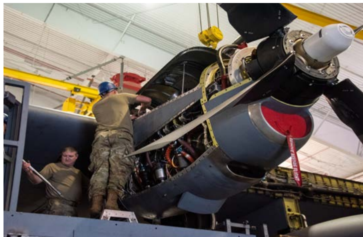
Airmen with the 166th Airlift Wing, 166th Maintenance Squadron, jet propulsion section, tighten a mounting bolt on a new engine at the Delaware Air National Guard Base, New Castle, Del., May 14, 2022. The original engine was removed from the aircraft as part of routine maintenance operations. Four bolts connect the engine to the wing, ensuring that the torque is correct is a critical part of the installation process. (U.S Air National Guard photo by Senior Airman Brandan Hollis)
