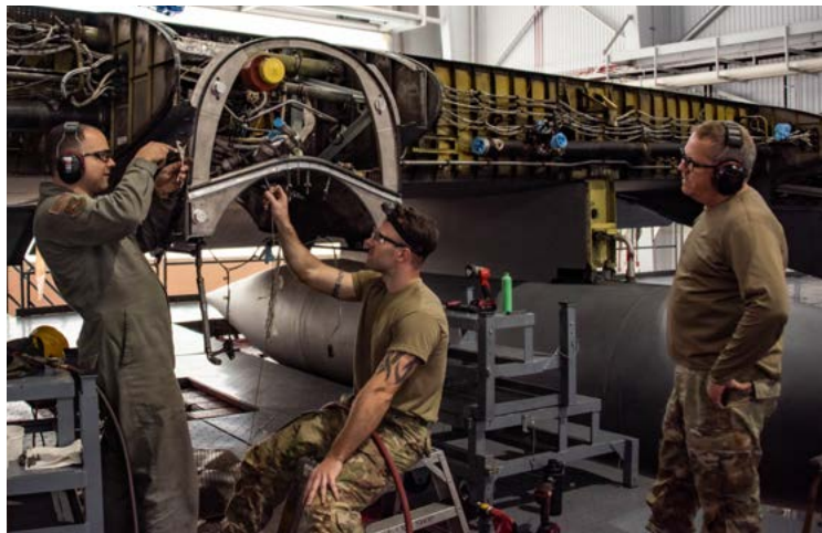
Airmen with the 166th Airlift Wing, 166th Maintenance Squadron fabrication shop inspect the engine truss mount for cracks before mounting a new engine at the Delaware Air National Guard Base, New Castle, Del., May 8, 2022. The original engine was removed from the aircraft as part of routine maintenance operations. (U.S. Air National Guard photo by Mr. Mitch Topal)
