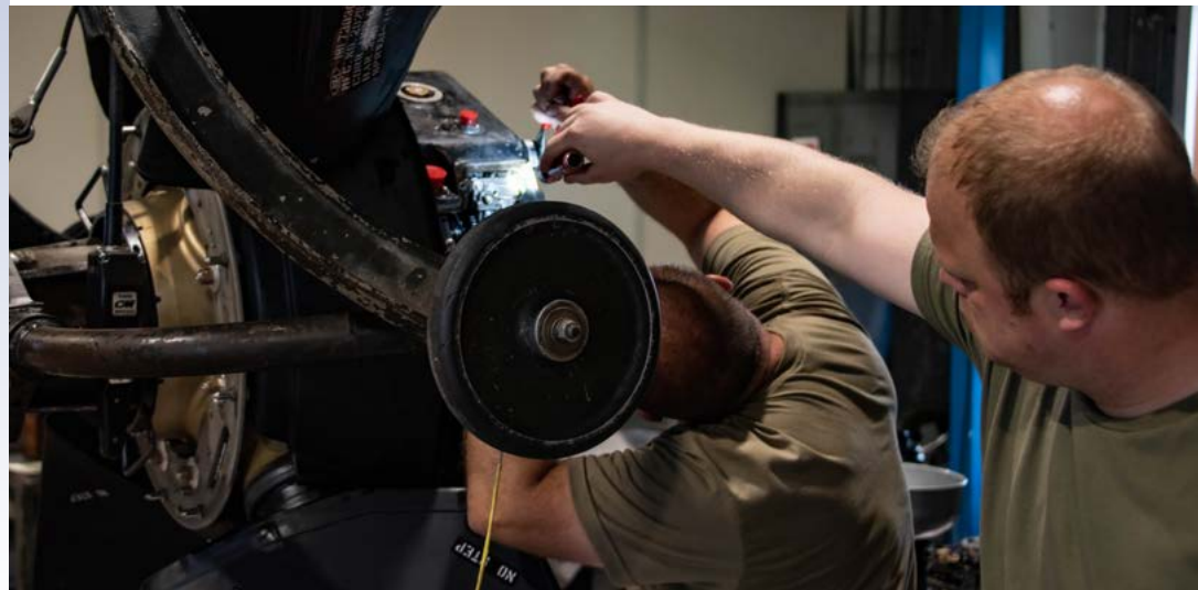
Propulsion Section Leaders MSgt Mark Wygant and TSgt Justin McGinnis, and Propulsion Technician TSgt Paul Freebery install a valve housing on to a pump housing for a propeller build up, 4-May-2022. This prop build-up was installed on a 166th Airlift Wing C-130H.2 during May RSD. (U.S. Air National Guard photo by Mr. Mitch Topal)
